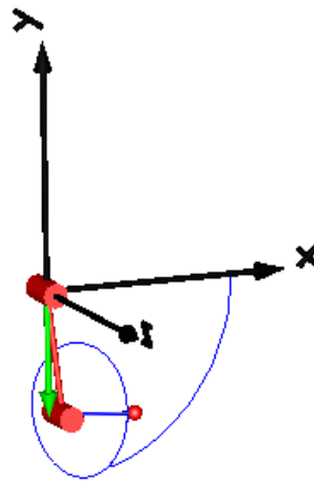
Figure 2.17: 3D visualization of the trajectory of the uncontrolled arm
